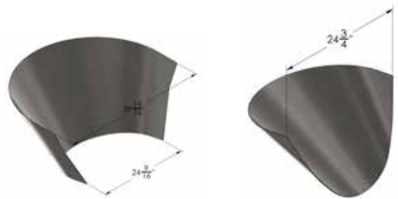
43650L-01 - CBMW Paver Upper Charge Hopper Liner 43650L-02 - CBMW Paver Lower Charge Hopper Liner
